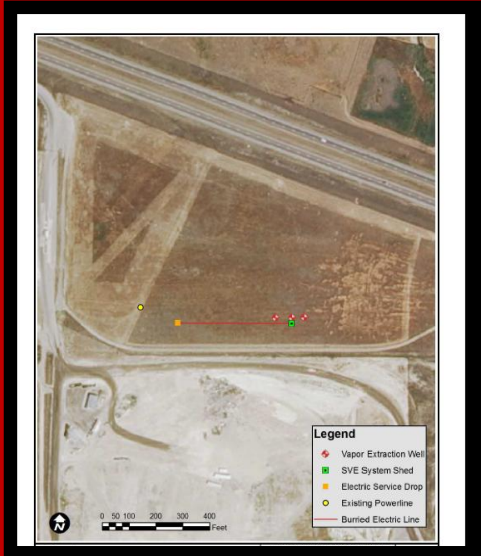
Olympus technical Services, Inc. Proposed SVE System Layout Logan Landfill
